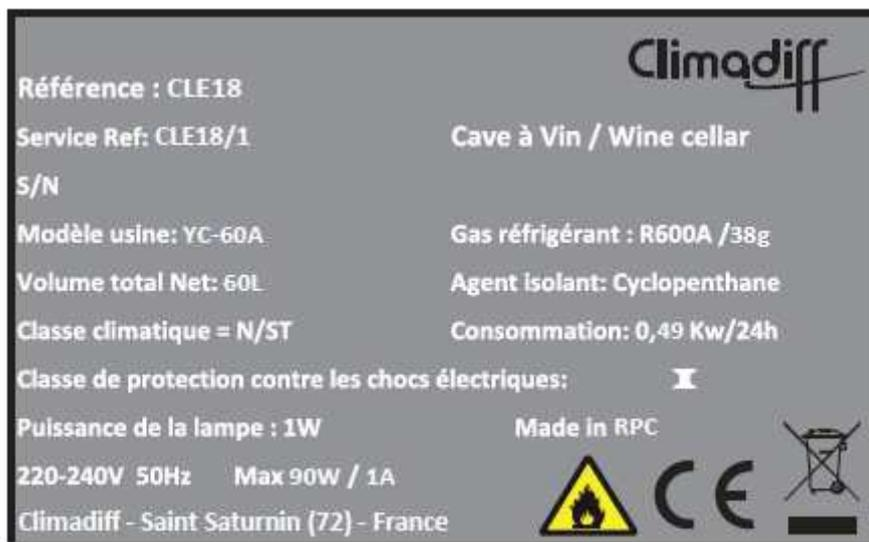
The nameplate attached to the inside or rear of the appliance (depending on the model) includes all the information specific to your wine cellar.
